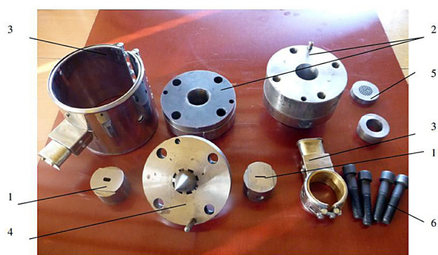
Fig. 2. View of the parts of extrusion head for profiles: 1 – die, 2 – body parts, 3 – annular heaters, 4 – distributive mandrel, 5 – filter of polymer
