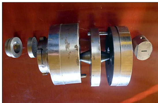
Fig. 2. View of the parts of extrusion head for profiles: 1 – die, 2 – body parts, 3 – annular heaters, 4 – distributive mandrel, 5 – filter of polymer
